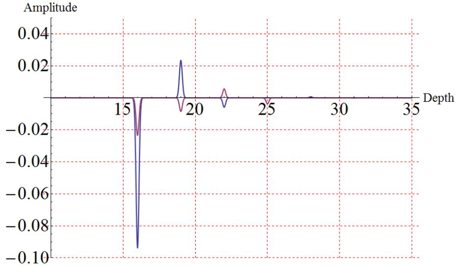
**Fig. 3.5a:** Comparison between  $D$  (blue) and  $D + D_3$  (purple). The comparison shows the contributions of  $D_3$  are (1) reducing the first-order internal multiples and (2) altering the amplitude of the higher-order internal multiples. Notice that, only internal multiples are plotted in  $D$ .
